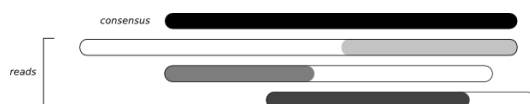
Figure 2. A contig resulting from prefix and suffix similarities, and its consensus sequence.
