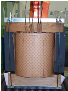
Fig. 2. Overview of 25 kVA single phase transformer.
