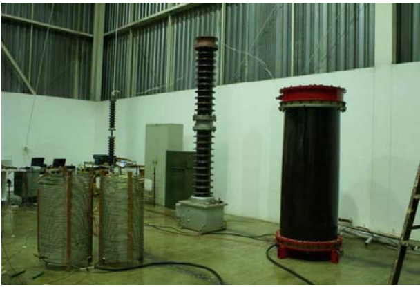
Fig. 12 – Calibration test setup at the lab – step-up transformer (at right), CVT (center), CVD (at left) and 1mH inductances used for reactive compensation (front)
