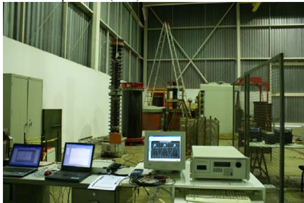
Fig. 13 - Calibration test setup at the lab – Power quality analyzer at left and arbitrary waveform generator, at right.
