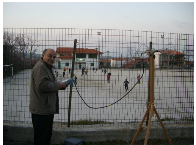
Fig. 8. Measurements of electrical field intensity in front of a school playground.
