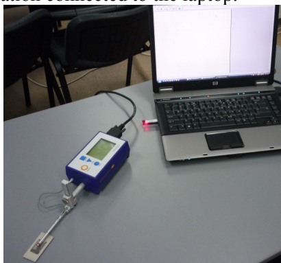
Fig. 5 Calibration of the roughness checker
