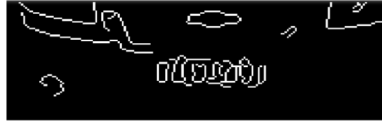
Fig. 2.3 Edge image of Canny operator filtering
