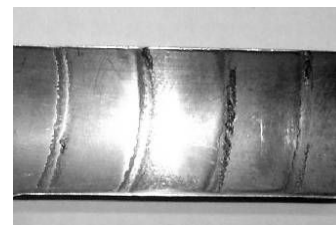
figure 8: discontinuities which are resulted during alternative stop and drawing of the pipe in the horizontal continuous casting process
