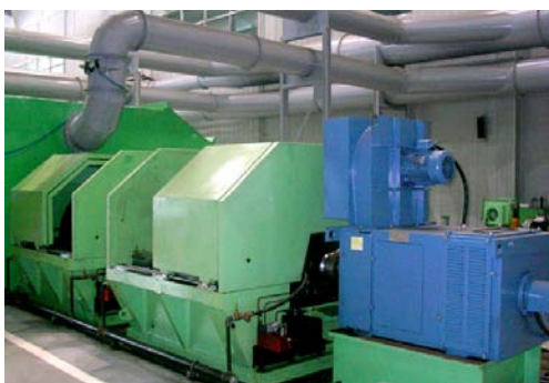
Fig.2 Brake performance dynamometer for high speed train
