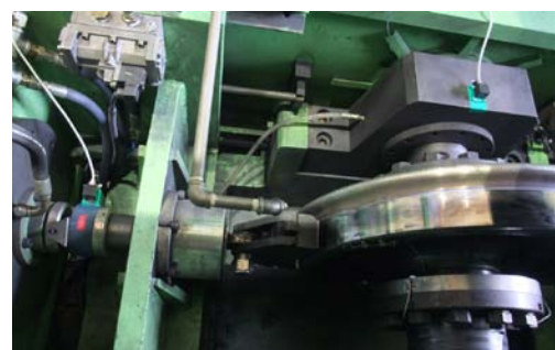
(a) Position of the 3-axis accelerometers
