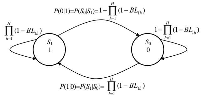
Fig. 2 A single-relay  $H$ -hop channel model.
