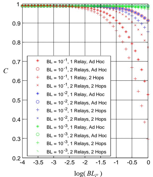
Fig. 4 The channel capacity versus the packet error probability in non-cooperative state for the number of relays and the number of hops as parameters.
