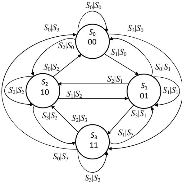
Fig. 3 Two-relay four-state channel model.
