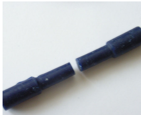
Fig. 9. The two wax halves ready to be attached
