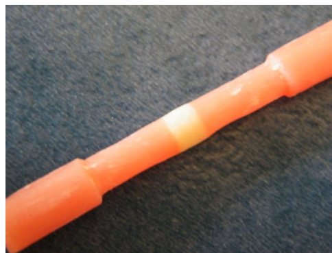
Fig.12. The tensile sample shape in accordance with ADA Nr.15
