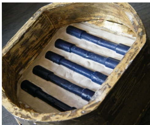
Fig.10. Wax sample mould patterns manufacturing process.
