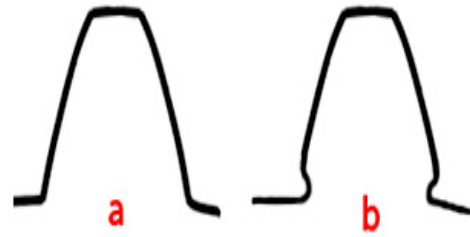
Fig.2 – Example of teeth profile: a) without and b) with geometrical error
