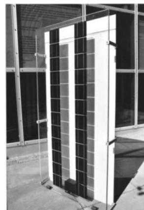
Fig 10. Wall integrated bifacial PV panel [10]
