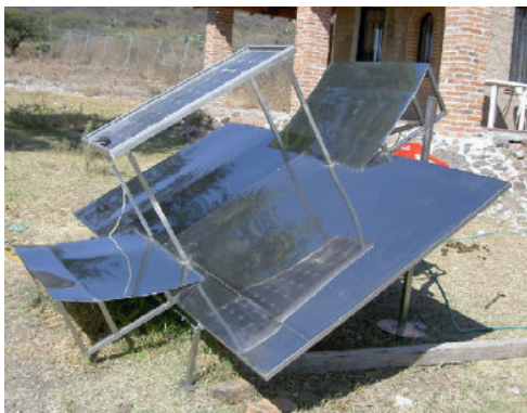
Fig 7. 1X bifacial PVT solar collector [8]
