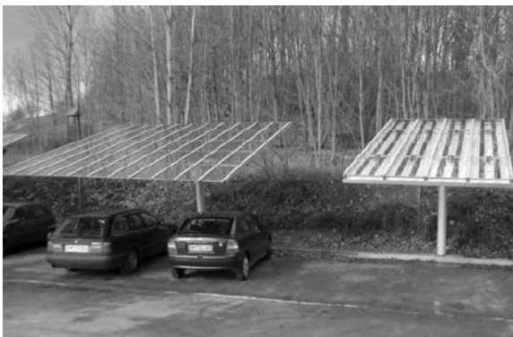
Fig 12. Parking lot integrated bifacial PV panel [10]
