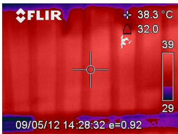
Figure 9: Captured image on the back surface of PV module with connected water pump
