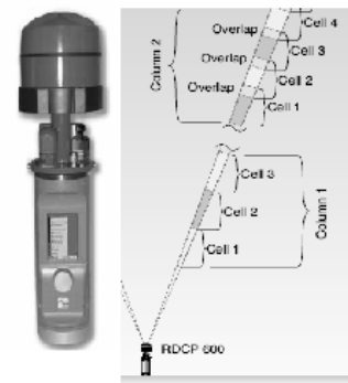
Fig. 5. RDCP600 Doppler current profiler
