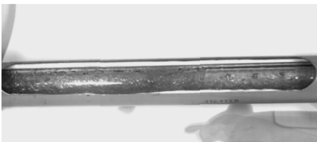
Fig. 7. Snapshot of the oil air mixture flow in the horizontal pipe section
