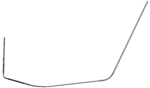
Figure 1: Three dimensional view of the geometry model of the scavenge pipe.
