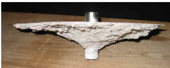
Fig. 2 Tensile loading – concrete-cone failure: illustration of the actual failure
