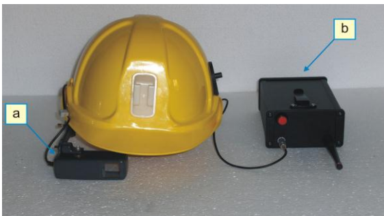
Fig. 7 (a) – AR display, (b) – navigation computer
