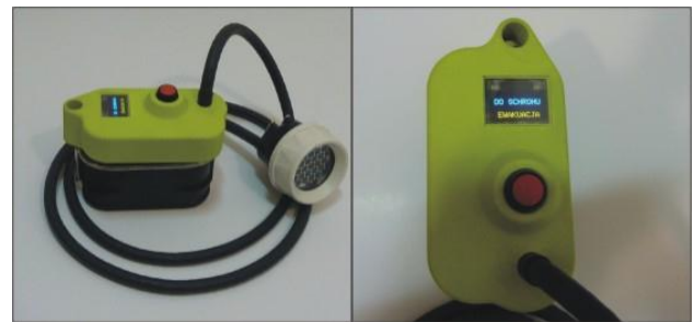
Fig. 3 Cap lamp with integrated location tag
