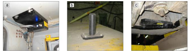
Fig. 5 (a) – vehicle tag, (b)- robust antenna (c)- RFID reader
