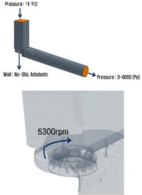
Fig.3 Boundary conditions and fan rotating speed
