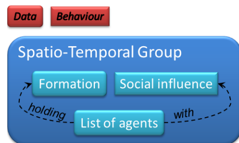
Fig 4: The spatio-temporal group (STG) architecture. A STG contains a list of the participating agents, as well as the geometrical formation they have to maintain and the social influence behavior they adopt.
