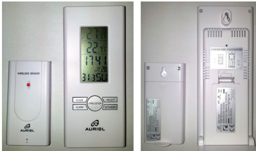
Fig. 5. Front and back view of wireless weather station Auriol type Z31055A-RX with radio sensor
