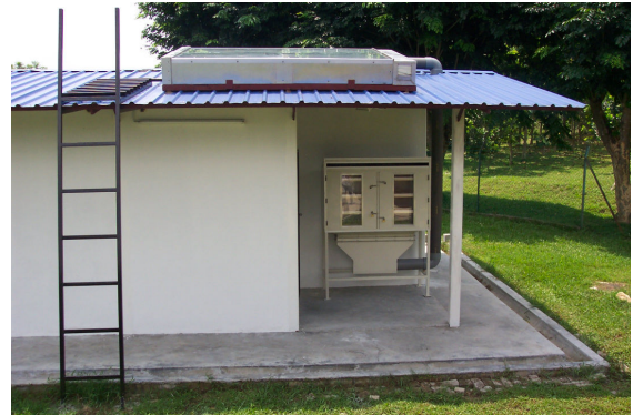
Fig. 18. The photograph of the solar dryer using double-pass solar collector with photovoltaic solar thermal collector
