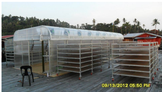
Fig. 10. The photograph of hybrid V-groove technology and solar house dryer for seaweed
