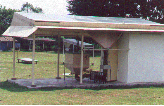
Fig. 14. The photograph of solar dryer using double-pass solar collector with integrated storage system
