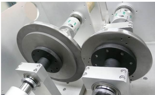
Fig.2 Specimens of wheel and rail for the scaled adhesion test-bench
