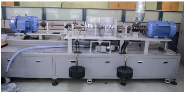
Fig.1 Scaled adhesion tester for analyzing the adhesion characteristic
