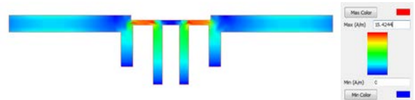
Fig. 9. Current flow visualization of generalized Chebyshev lowpass filter at 6 GHz
