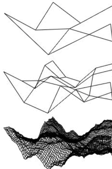
Fig. 9 Fractal terrain generation using Diamond-Square algorithm by David P. Feldman (2012) [8]
