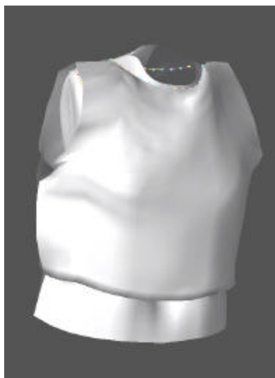
Figure 12: Sample 1 with higher Bending Stiffness in Weft Direction
