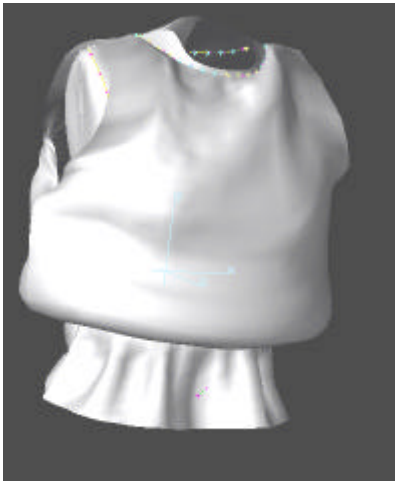
Figure 11: Sample 1 with lower Bending Stiffness in Weft Direction
