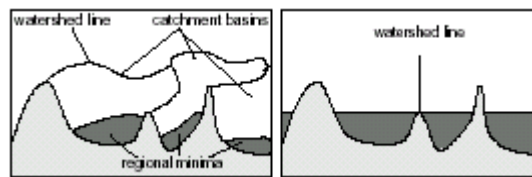
Fig. 1: The topographic analogy: points where two lakes meet define the watershed line.
