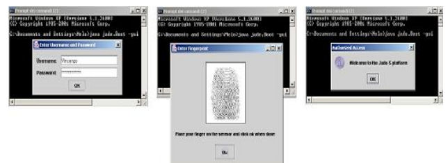
Fig.9: In the figure is shown the whole access platform procedure. In (a) the first security level with username/password requesting is shown; in (b) the second security level with the user fingerprint requesting is shown; finally in (c) a welcome access window is shown.
