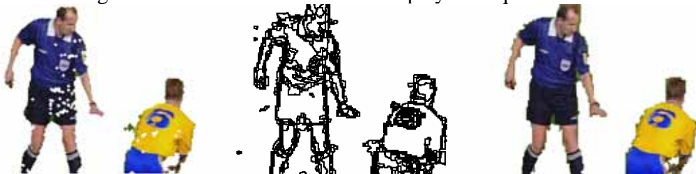
Fig. 7 : (a) is result of temporal segmentation , (b) is result of spatial segmentation , and (c) is the extracted object.
