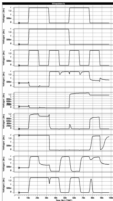
Figure 6: Simulated waveforms of 16-t full adder [5] at V_{DD}=2V (wrong results)
