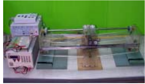
Fig. 7 The practical hardware structure of the seesaw system.
