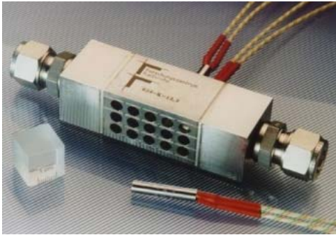
Fig. 1. Electrically heated micro heat exchanger.
