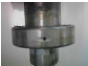
Fig. 5: Bearing with a hole in the outer race
