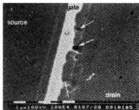
Fig. 26 ESD damage occurs at NMOS gate [35] .
