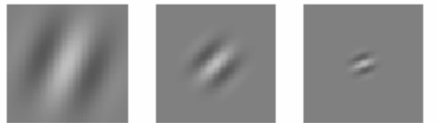
Fig.4. Real components of Gabor wavelet filters at different orientations and scales.
