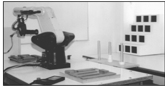
Figure 3. Elements of the vision system (robotic arm CRS A465, CCD camera and calibration object).
