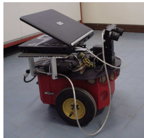
Figure 6: The mobile robot with stereo head.
