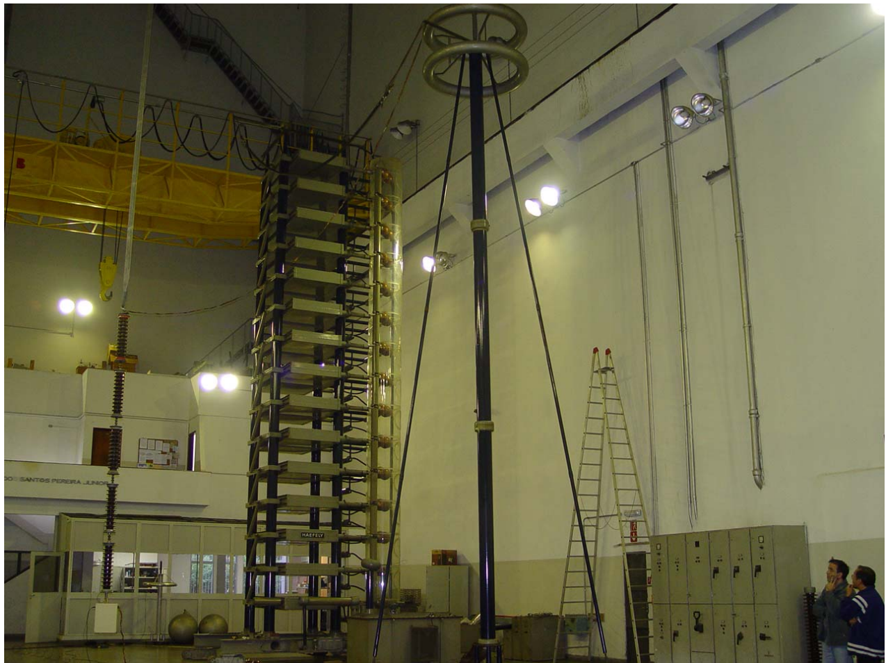
Fig. 12 Laboratory setup for the switching transients tests, showing the capacitive divider (at left), impulse generator (center) and the reference divider (at right).
