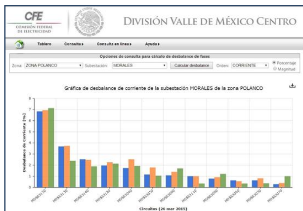
Fig. 17. Feeders Phase Unbalance for a Substation.
