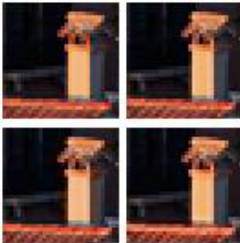
Top left: Original image; Top right: The 4:2:2 image subsampling; Bottom left: The 4:1:1 image subsampling; Bottom right: The 4:2:0 image subsampling
