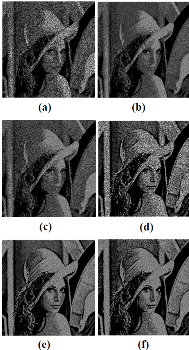
Figure 2: Comparison between applying the unsharp mask for SI (the second row) before using methods P-SVICS, ME-SIVCS-1, ME-SIVCS-2 and using methods without applying the unsharp mask (the first row): (a) P-SVICS, (b) ME-SIVCS-1, (c) ME-SIVCS-2, (d)-(f) are P-SVICS, ME-SIVCS-1, and ME-SIVCS-2, respectively, after the unsharp mask was applied on SI.
