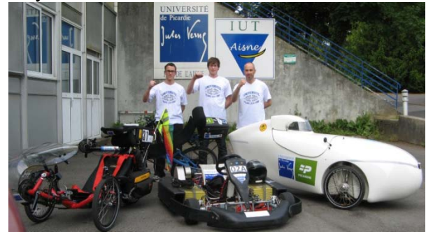
Fig. 7. Different prototypes of electric vehicles (Left to right) bent rider, tricycle, go kart, velomobile.
