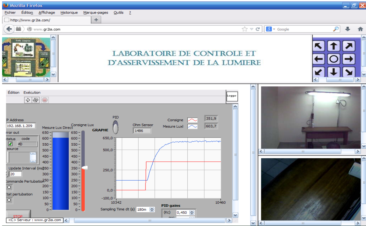
Fig. 6 Open loop step response under disturbance (125 Lux)
