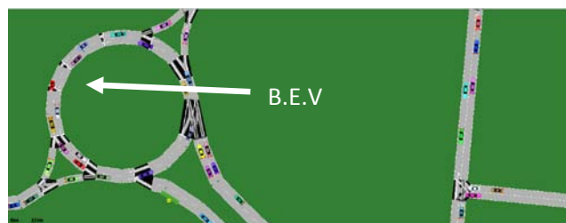
Fig. 6. Snapshot of SUMO simulation showing the target vehicle (BEV)
