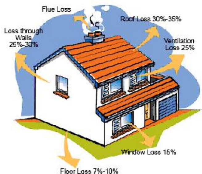
Fig 6: Heat Loss of a building.
