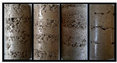
Fig. 5a: Mixing water content effect on homogeneity of specimens
