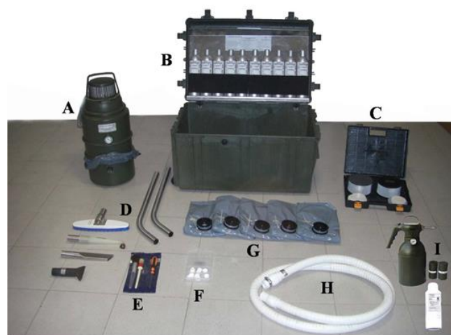
Fig. 3 - SX34 decontamination equipment prototype. A. Deco vacuum aspirator (9.5 kg - 20.9 lbs; 220 ÷ 240V – 50 ÷ 60HZ; 1200 W); B. Chest container and 10 canisters (capacity 0.75 l each) of SX34 decontaminant; C. HEPA and ULPA filters; D, H. Accessories and connections tubes; E. Brushes and maintenance accessories; F. Nozzles; G. Bags for the collection of contaminated materials; I. PSDS/1,5 MIL decontamination system-acids resistant according to STANAG 4360.
