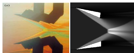
Fig. 5: Comparison of our results ( \theta_1 = 28.44^\circ , \theta_2 = 24.14^\circ ) (right) with the work [1] ( \theta_1 = 28^\circ , \theta_2 = 24^\circ ) (left), under the same conditions. M_0 = 4.96 .
