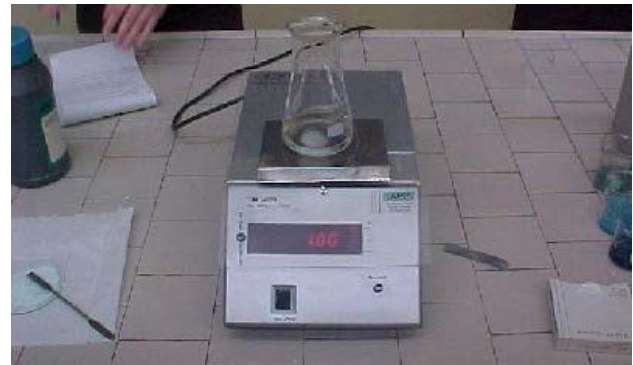
Fig. 2. Solute concentration of CMC-water solutions is set by using precision scale and a 250-ml flask.
