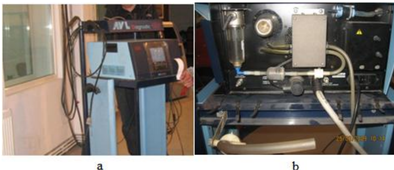
Fig. 3 Dicom 4000 gas analyzer a - analyzer image; b- measurement sensors
