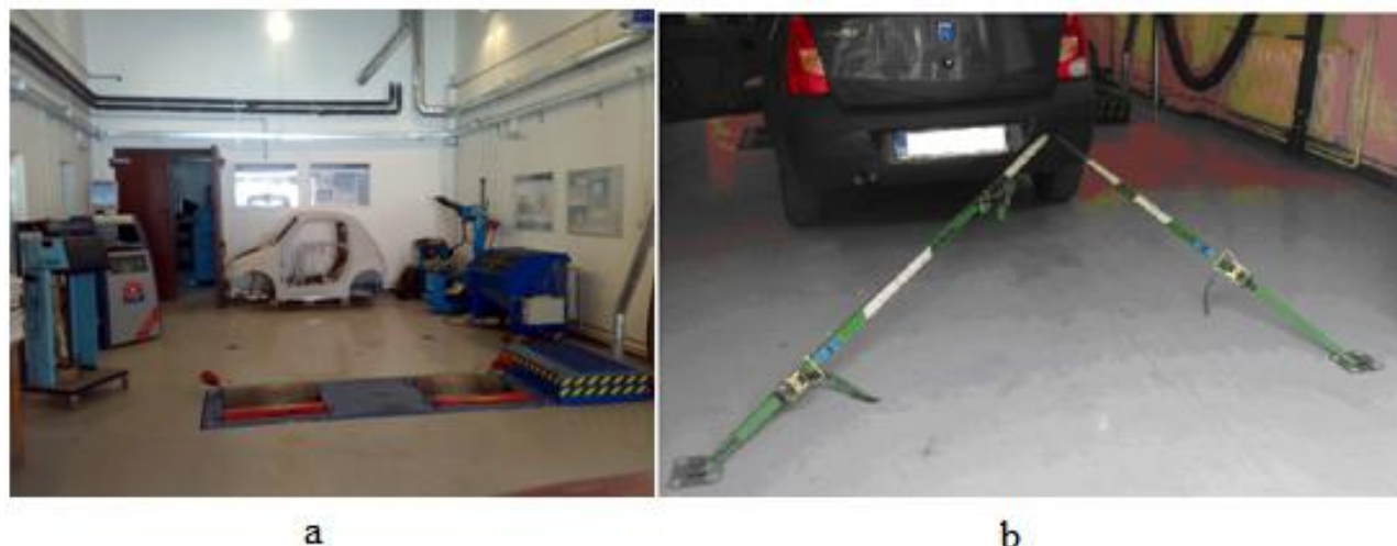
Figure 2 Experimental stand a - testing equipment, b - vehicle positioning on the chassis dynamometer
