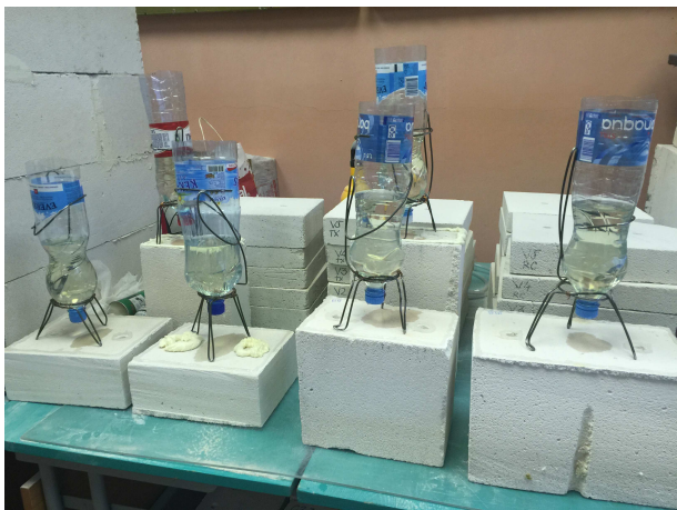
Fig.4. Stand of the water application on the AAC masonry blocks in condition of water droplets
