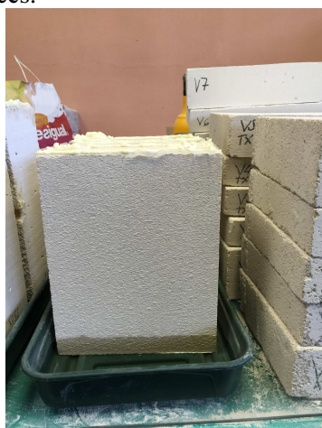
Fig.1. Monitoring of water infiltration in AAC masonry block
